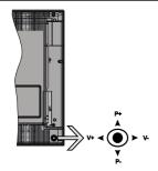
The joystick allows you to control the Volume / Programme (while watching TV channels) / Source and Standby-On functions of the TV.
